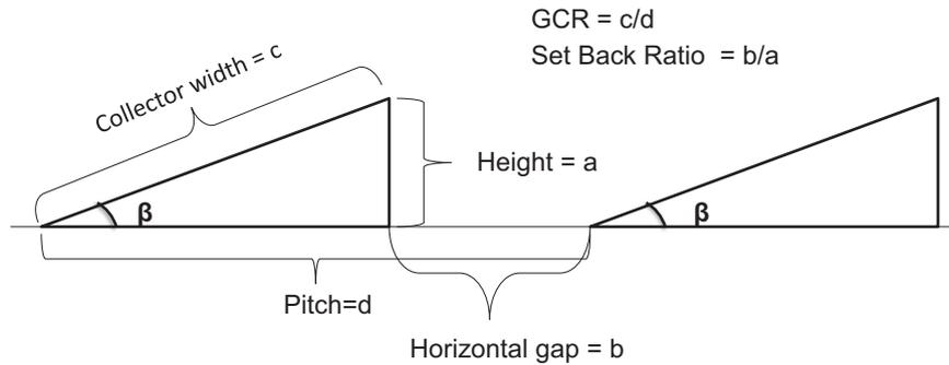
**Fig. 3.** Ground Coverage Ratio (GCR) calculations and dimensions [98].
