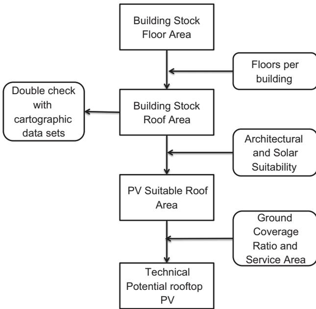
Fig. 5. Step-by-step overview of the proposed methodology.
