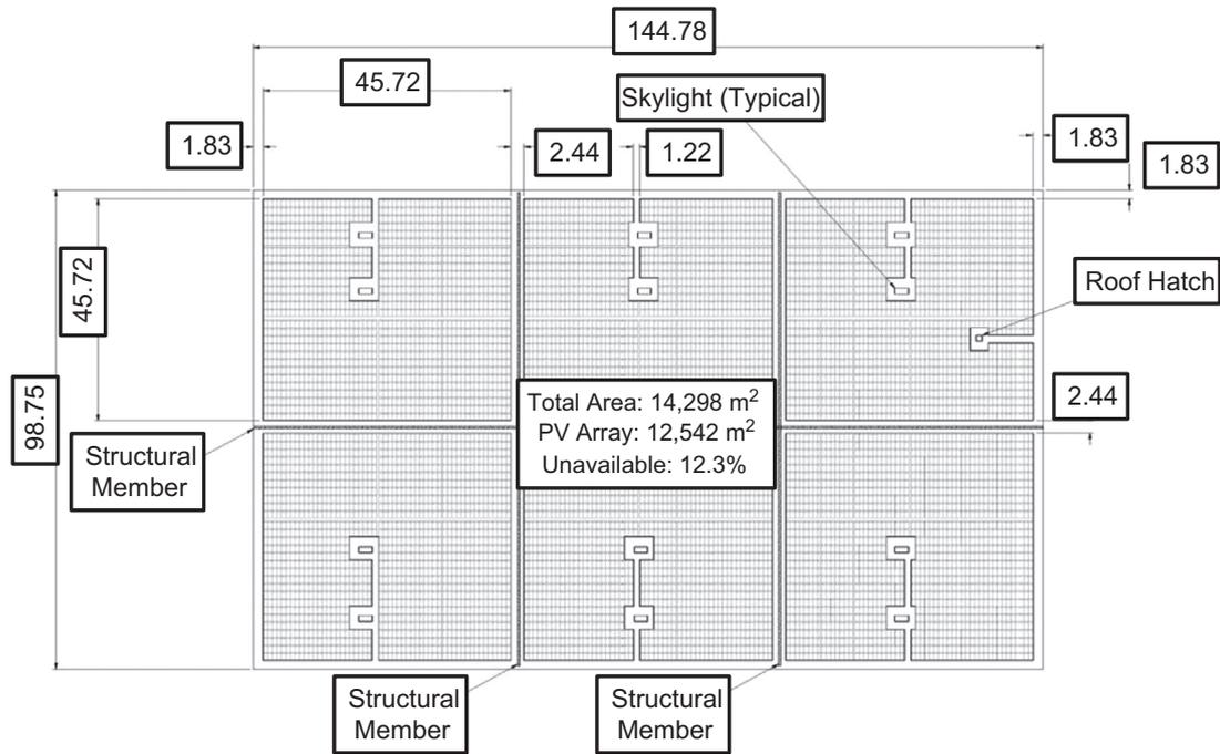
Fig. 4. Schematic illustration of a no-tilt PV system on a large commercial rooftop. Units in meters. Adapted from [98].
